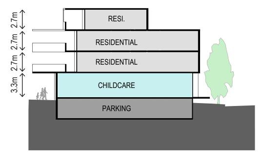
FIGURE 8. CEILING HEIGHTS SECTION THROUGH BUILDING D
