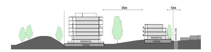
FIGURE 2. BUILDING SEPARATION IN SECTION
